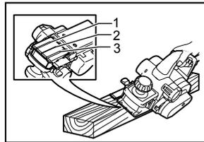
1. V groove (medium amount of chamfering)
